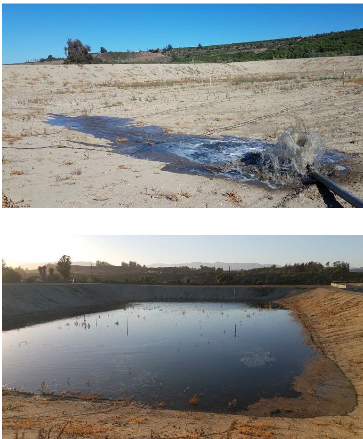
Figure 14. Pond 9 water application of 230k gallons (0.85 AF) at start (top) and after full (bottom).
