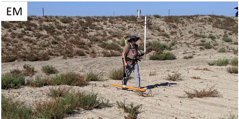
Figure 3. Characterization methods include EMI (EM photo), ERT, DTP, and modified seepage meters for infiltration tests.
