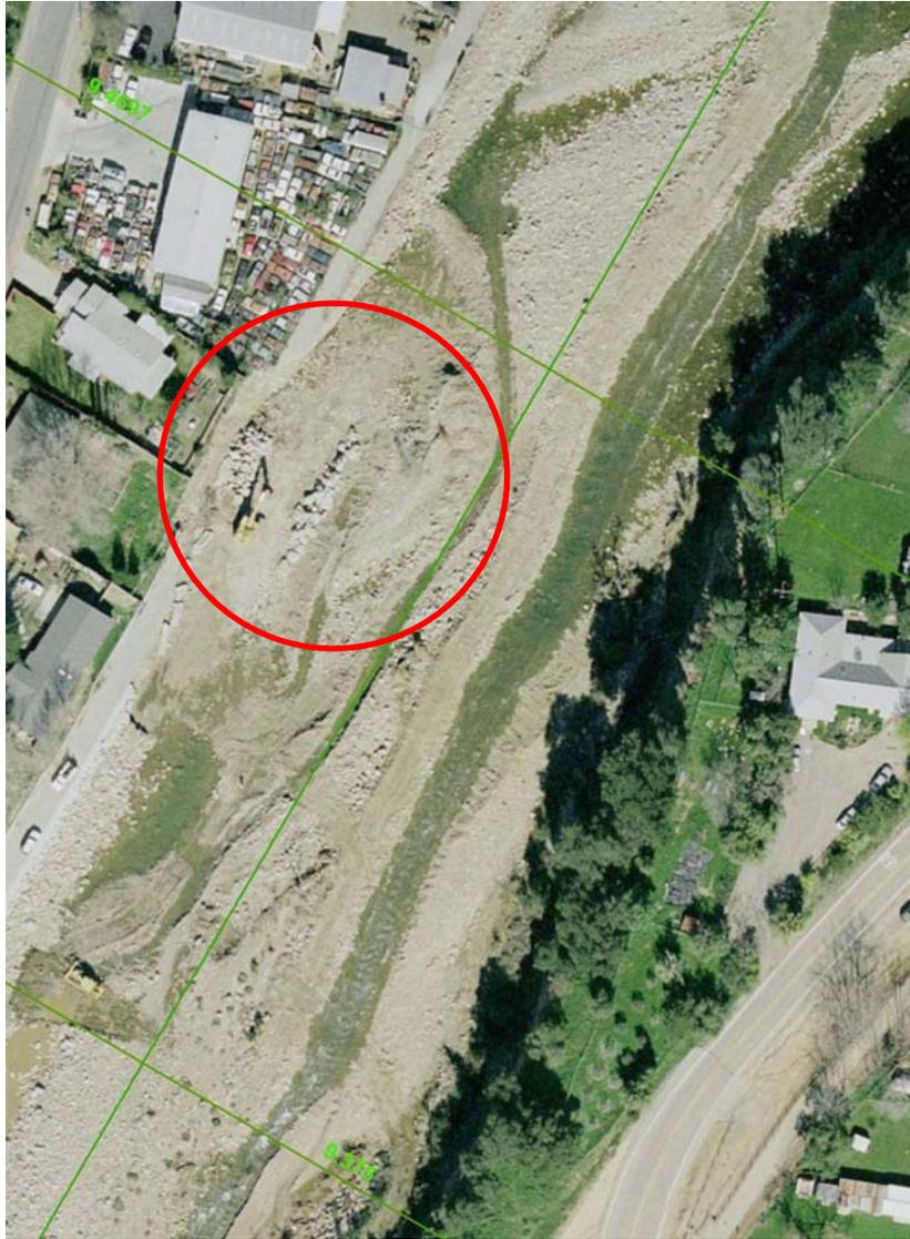
Figure 4.12. Aerial photo taken in February 2005 showing erosion of Live Oak Levee between XC 9.375 and 9.4697.
