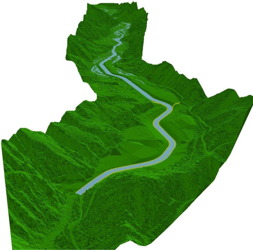
Figure 7.1. Oblique View of Channel Immediately after Dam Removal.
