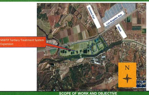
Construction of the Tertiary system including but not limited to additional filter modules, chlorine contact tank expansion, new baffle walls, RAS/WAS pumps, yard piping, electricals, instrumentation and controls, and recycled water storage facitity.
