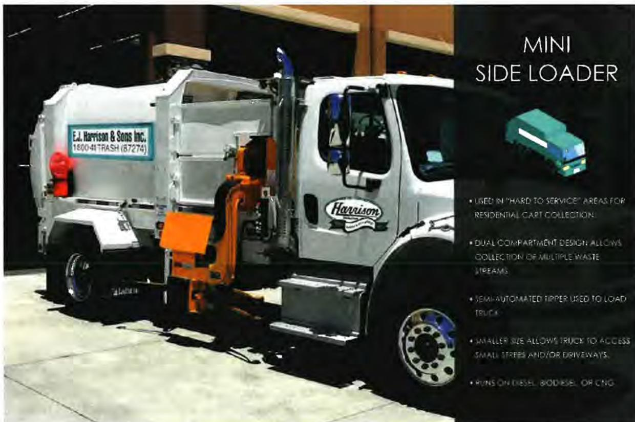
These smaller trucks are better equipped to accommodate private streets, driveways and alleyways that are typical in large, rural settings. The driver needs to exit the vehicle and bring the cart to the tipping mechanism on the right side of the vehicle, where the driver will engage the tipping mechanism
