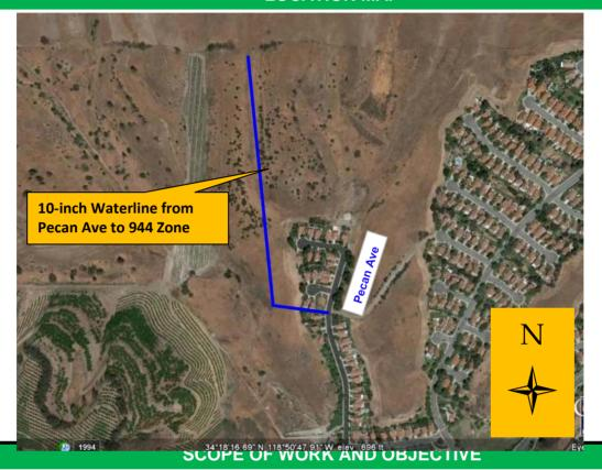
Install approximately 3,500 lf of 10-inch water line to connect 944 and 1180 pressure zones per Master Plan and to improve operational flexibility in the system.
