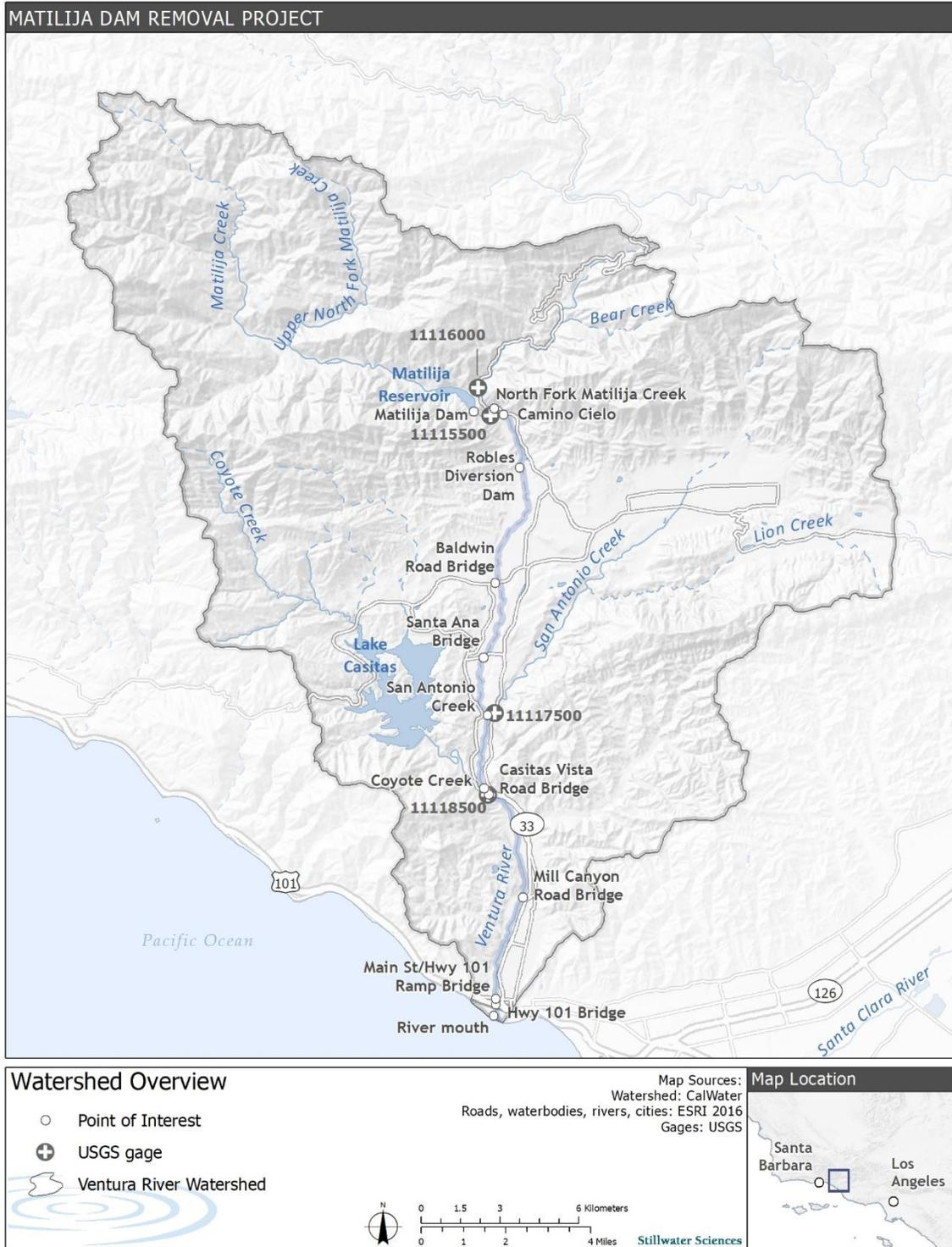
**Figure 1.** Map of the Ventura River watershed (modified from Figure 2.1 of BOR 2006), showing the major crossings of the river and the four USGS gaging stations used for sediment transport modeling.
