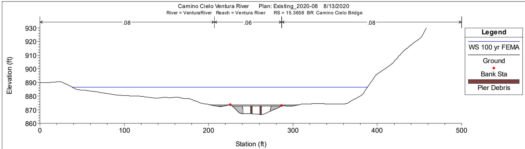
**Figure 5. Pre-Bridge Project (Existing Low Water Crossing) Cross Section**
