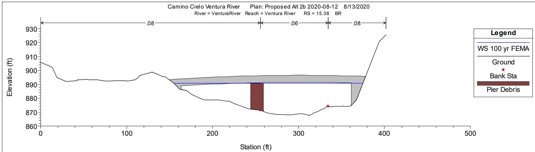
**Figure 6. Post-Bridge Project (Proposed Bridge) Cross Section**
