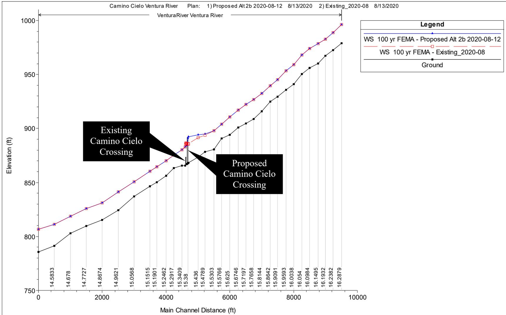
**Figure 4. 100-year FEMA Flow Water Surface Profile Comparison**
