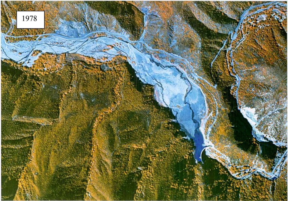
**Figure 3.-- Matilija Reservoir in 1978. Note dam in lower right of frame, very small remnant of reservoir pool. Photograph by "Pacific Air", supplied by EDR, Inc's. aerial photo database search.**
