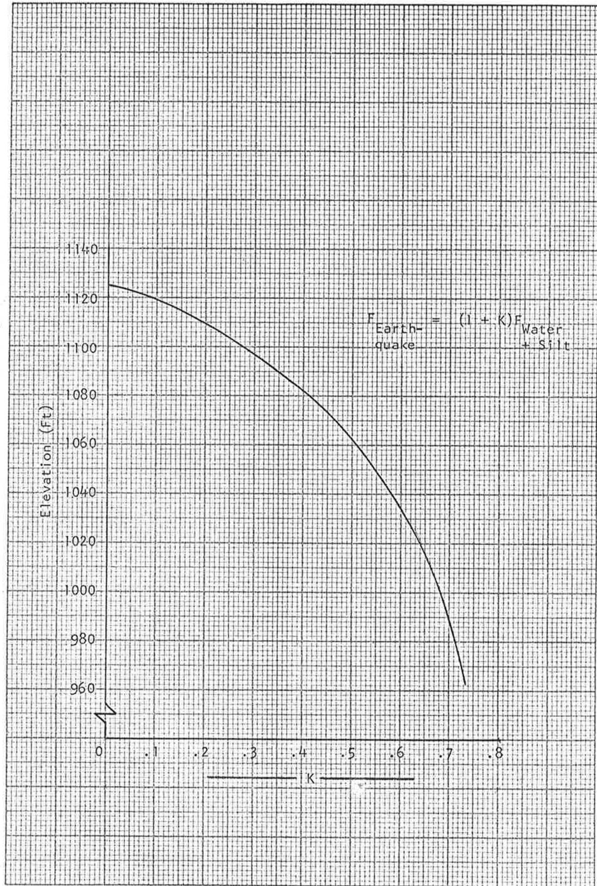
FIG. 4.1. Incremental Increase in Hydrostatic Pressure Due to Earthquake
