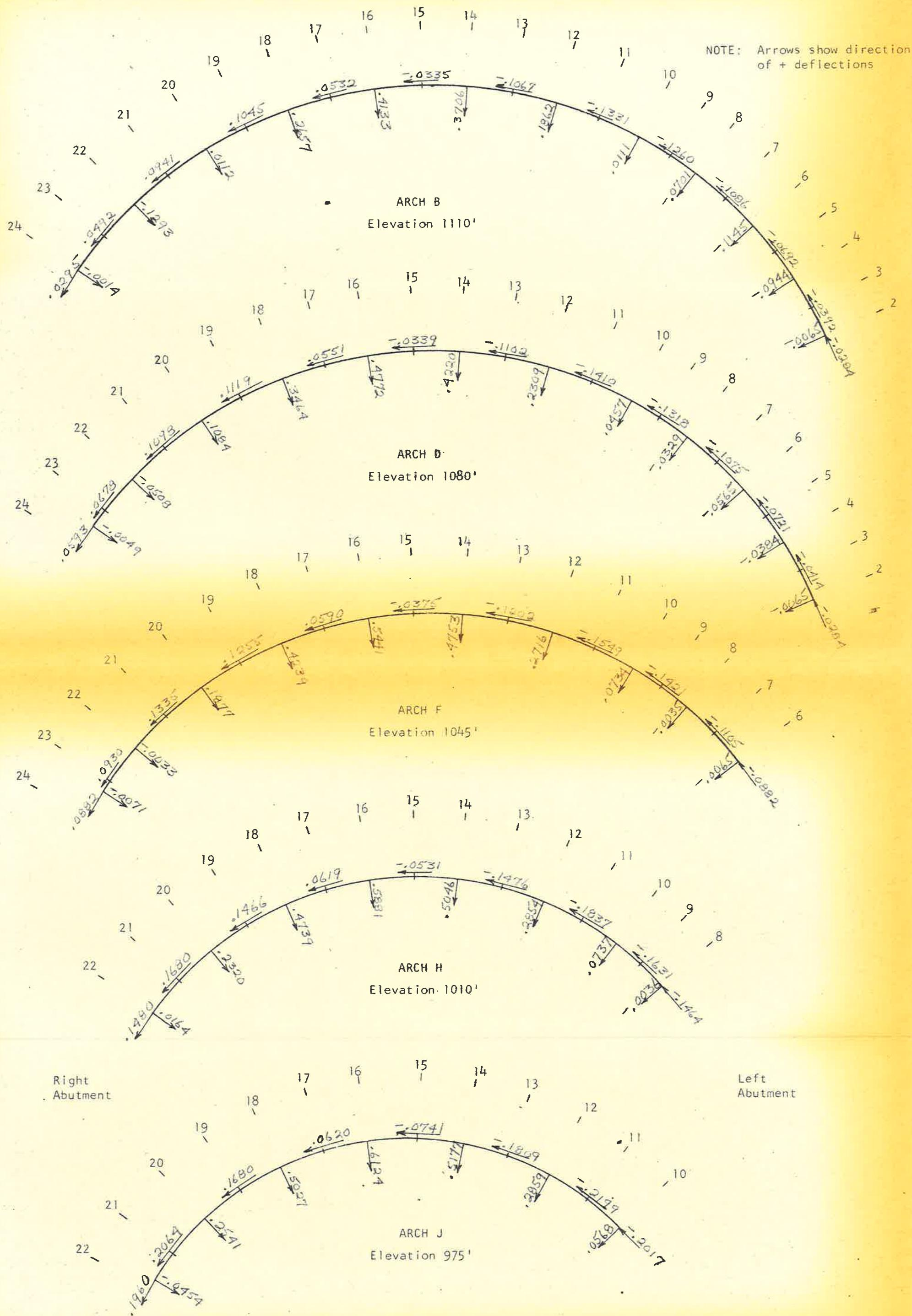
Load Condition B+E, Water Elevation 1069, Silt Elevation 1037
