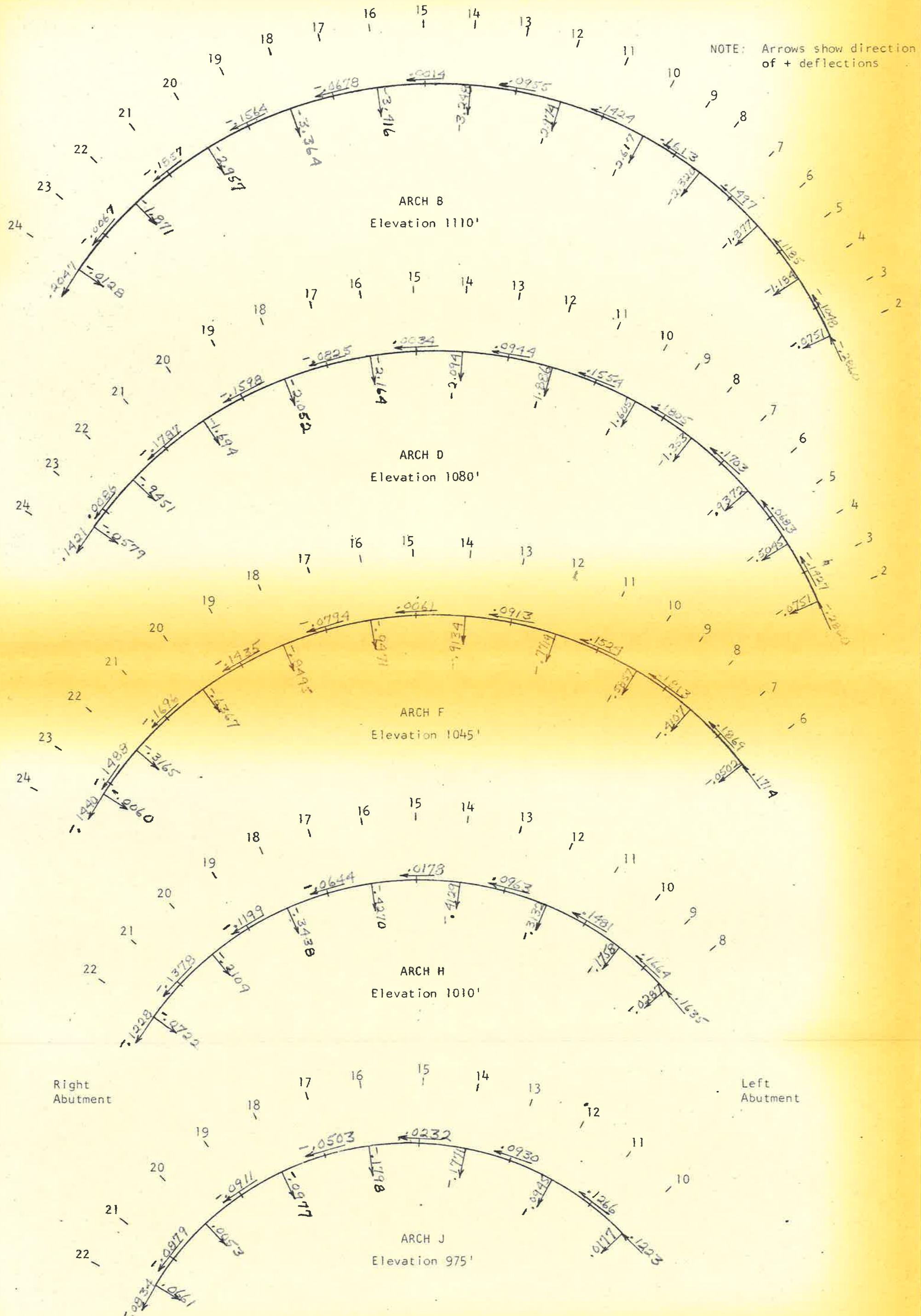
Load Condition K, Chemical Expansion; 0.1% Above Elevation 1062.5
