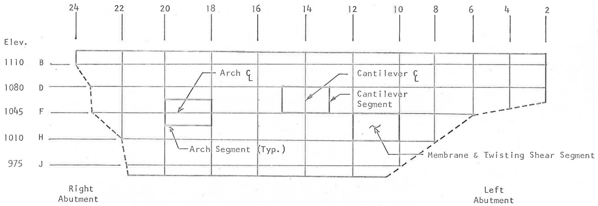
FIG. 2.4. Lumped Element Identification
