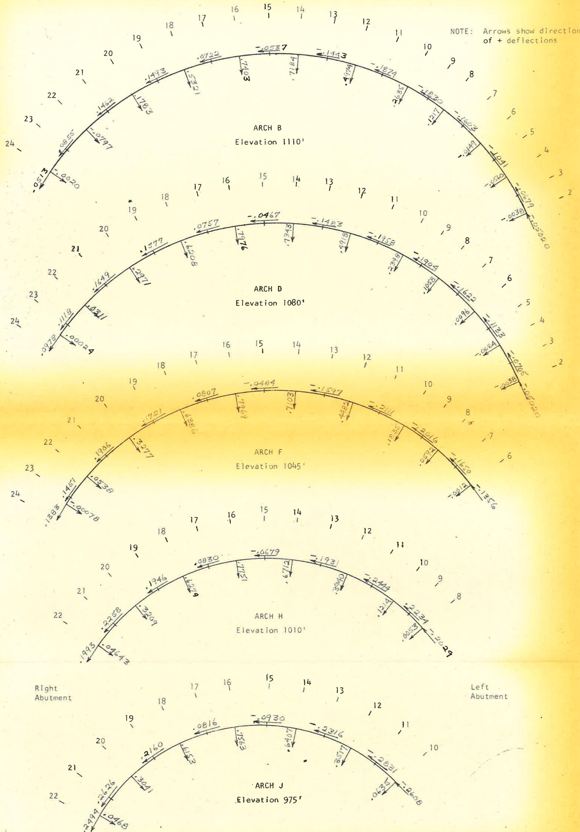
Load Condition A, Water Load Only, Elevation 1103
