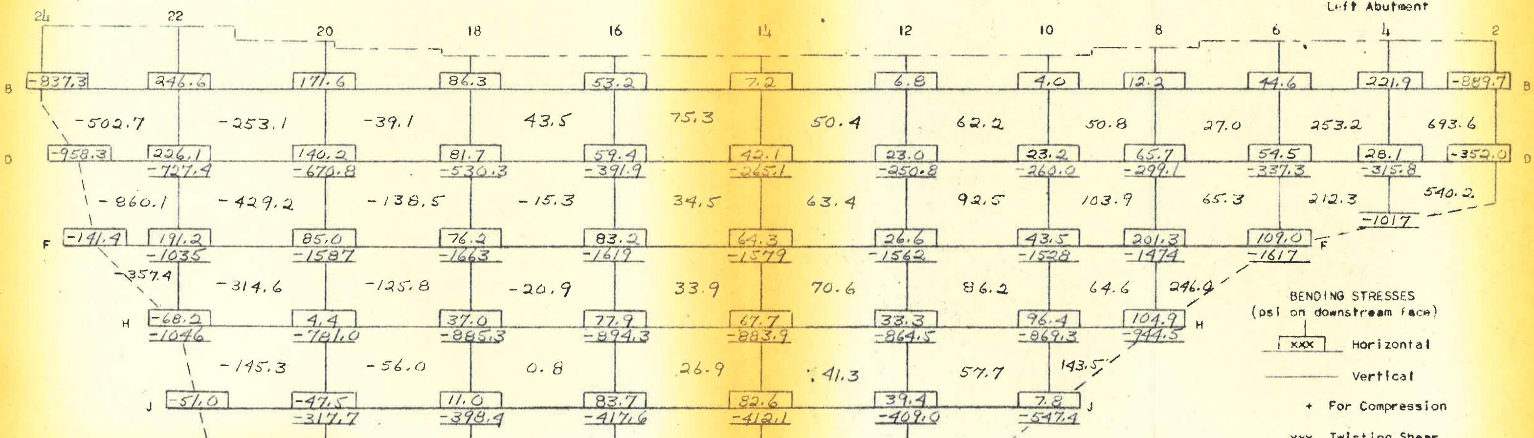
Load Condition K, Chemical Expansion: 0.1% Above Elevation 1062.5
