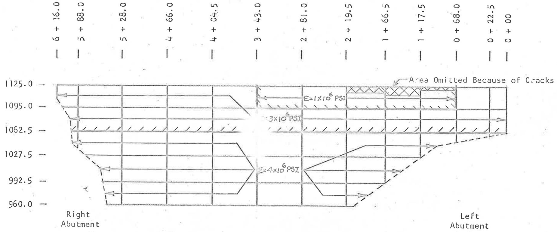
FIG. 2.5. Modulus of Elasticity of Analytical Model
